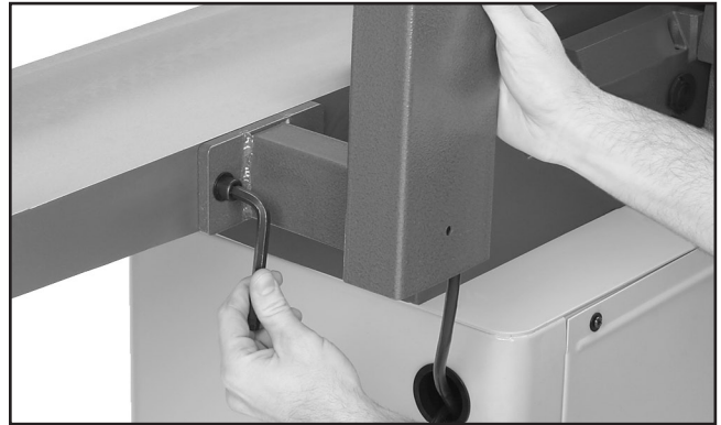
Figure 15. Attaching pedestal switch to stand.
